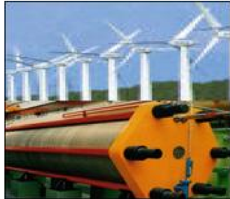
Electrolysers working with electricity from wind energy
